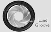
With a rifled bore, you can use cylindrically shaped ammunition. This has two advantages: the mass of a cylinder is greater than that of a sphere of the same diameter, and a cylinder has a larger surface for a faster spin. A faster spinning, heavier bullet has greater range, accuracy, and impact.
