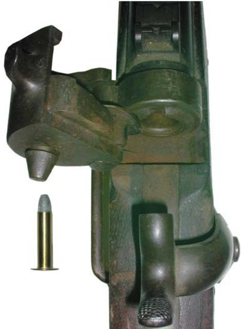
The Joslyn Model 1861 .54 caliber carbine had a hinged block over the breech (above) to load a brass, centerfire cartridge. From the collection of Cordy Rich, photos by Gerry Stoner, courtesy of Cordy Rich.
