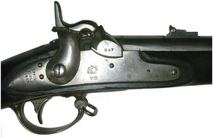
The Model 1832 Springfield musket was converted to a caplock sidearm for the army at Harpers Ferry (left). The breech was modified to accept a cap head, the flintlock was removed, and a new caplock (above) from Hewes and Phillips was installed. From the collection of Cordy Rich, photos by Gerry Stoner, courtesy of Cordy Rich.
