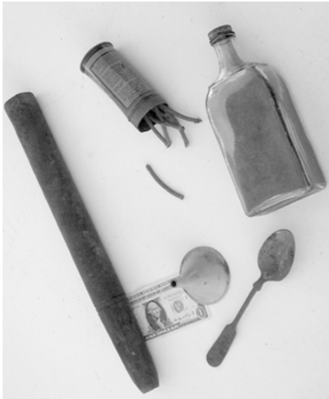
The splitting gun, fuses, funnel and spoon, and a jar of black powder with the dollar bill shown for size. Courtesy of Carlton Lewis, photo by Gerry Stoner.
